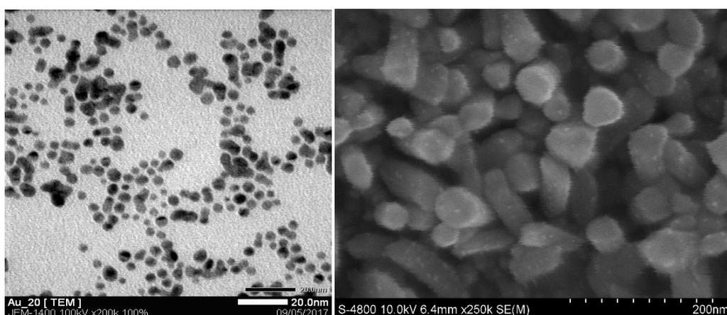
**Fig. 4: (a) TEM of Au NPs in solution after hydrothermal process and (b) SEM of the ZnO nanorods modified by Au NPs**
