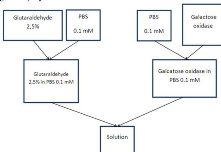
Fig. 1: Flow chart for the immobilization galactose oxidase on ZnO nanorods surface
