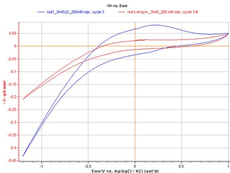
**Fig. 5: The CV curve of (a) the pure ZnO nanorods and (b) the immobilized ZnO nanorods in 200 mM galactose solution**
