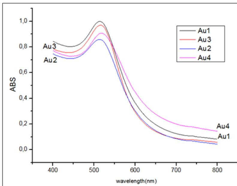
**Fig. 3: The UV-Vis spectrum of solution after hydrothermal process with different hydrothermal time (from 1 hour to 4 hours - sample A1 to A4)**
