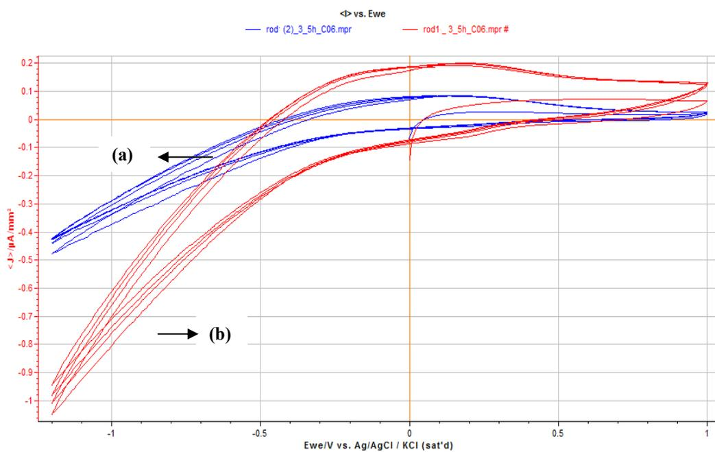
**Fig. 6: The CV curve of (a) the GOx|ZnO|FTO and (b) the GOx|Au-ZnO|FTO in 200 mM galactose solution**
